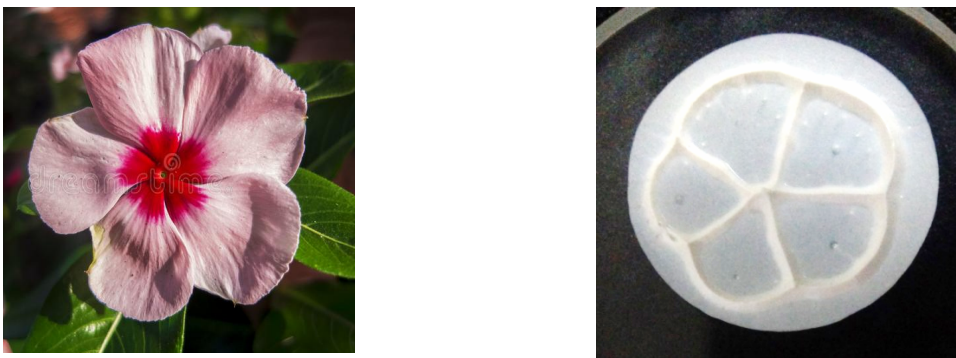
Figure 12: Replicating flower petals structure using the centroidal hole mechanism.
